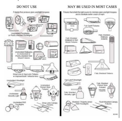
The lights on the left are non-conforming. Those on the right can be used in most cases. Depending on the mounting height and proximity to the property line, additional shielding may be necessary to prevent the luminous elements from being visible from any other property.
